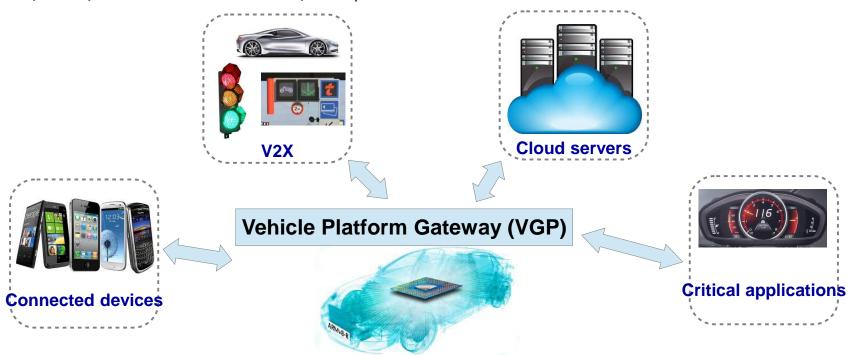
VGP must support interconnection with external applications while ensuring in-vehicle buses secure access to ECUs, which contains critical applications
